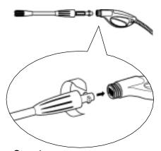
Step 4 Slide the spray wand extension into the gun. Turn the wand collar clockwise onto the gun threads until tight.
